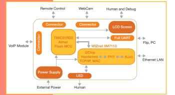
with Atmel 80C51 Flash MCU and the WIZnet i2Chip<sup>®</sup>, a unique hardwired embedded Ethernet TCP/IP chip. The customer can change functions and reload firmware using In-System Programming capability. Error messages can be displayed on the LCD screen, allowing easy debug of user's application. After evaluation, the drop-in network module (IIM7010) supplied in the kit can be re-used.
